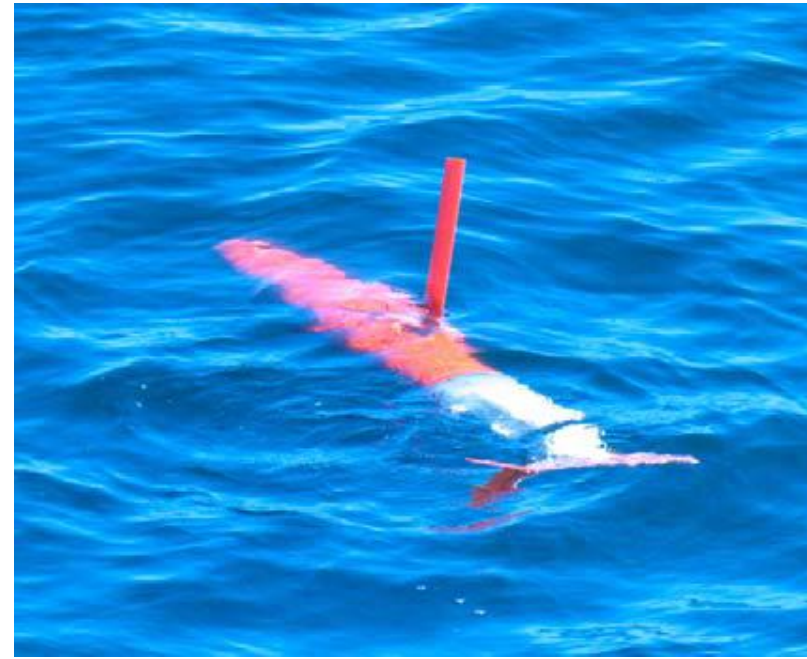
Figure 3. The Spray Glider inducing a roll to lift its wing out of the water to obtain a GPS fix.
