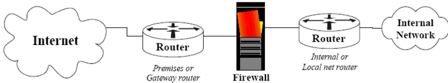
Two Router Firewall Configuration for a Network Boundary
